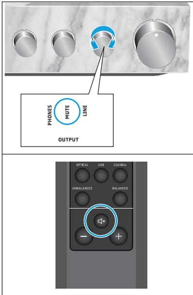
▷ Turn the **OUTPUT** rotary switch until **MUTE** points to the marking.
