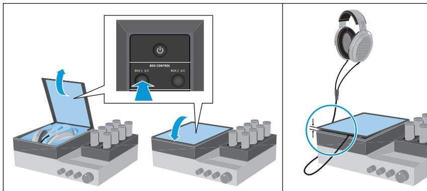
**i** If the **OUTPUT** audio output is set to **LINE**, the headphone storage boxes remain closed when the HE 1 is switched on.
