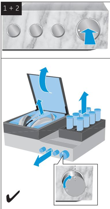
1. Set the power switch to **ON** to switch the HE 1 on.
