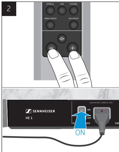
**i** When restoring the factory default settings, make sure to point the remote control at the remote control sensor located on the front bottom of the amplifier. Otherwise the amplifier switches on normally.
