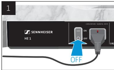
1. Set the power switch to **OFF** to switch the HE 1 off and wait until the status LED goes off (up to 30 seconds).
