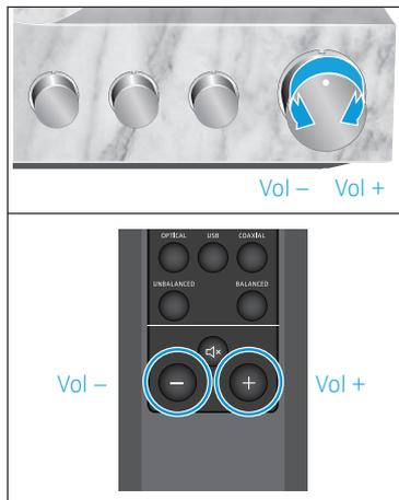
The volume setting applies to both the headphones (**PHONES**) and the audio outputs (**LINE**). If you have connected two headphones to the headphone amplifier, the volume setting applies to both headphones. The volume/signal levels of the INPUT audio input and OUTPUT audio outputs can be adjusted individually (see page 33 and 36).
