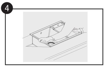
放置厨盆:将厨盆前缘紧贴台面开口处的前缘,再将厨盆缓慢放下。 Position sink by tilting back of sink up: Place front rim of sink close to front edge of sink opening, then lower back of sink into opening position carefully.
